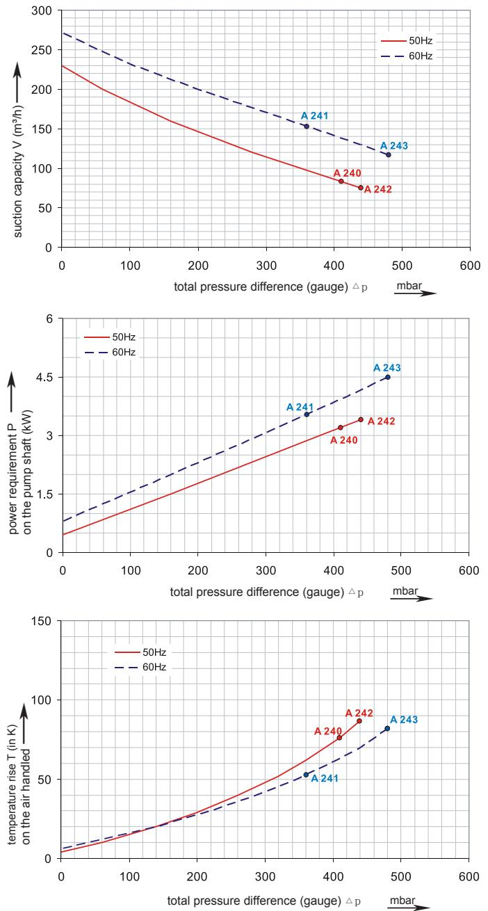
Each G-2RB type can be applied both as vacuum pump and compressor in continuous operation over the total stated performance curve range. The motors are available as standard for the input voltage range of 50 and 60 Hz and for protection category IP 55 as well as approved for UL and CSA.
